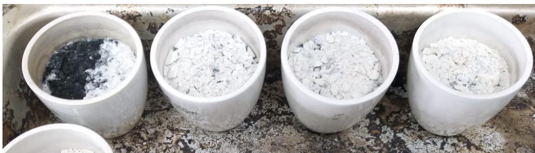
Figure 4. Visual appearance of the starch residue after muffle furnace burning
