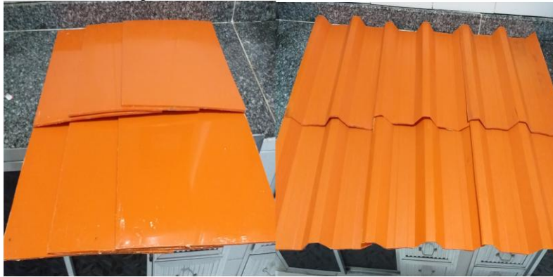
Figure 5. Photographs of sheets and tiles made from recycled HDPE
